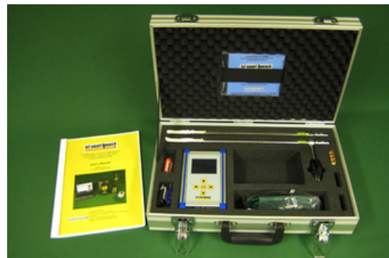
The data acquisition unit with accessories, the test probe with handle, a USB with the computer software and the manual are all contained in a carrying case.
